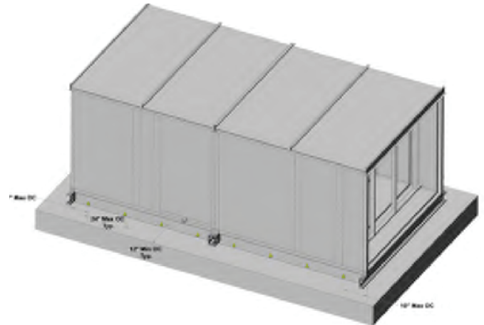
Figure 40: Unit with Base Frame Mounted on Concrete
